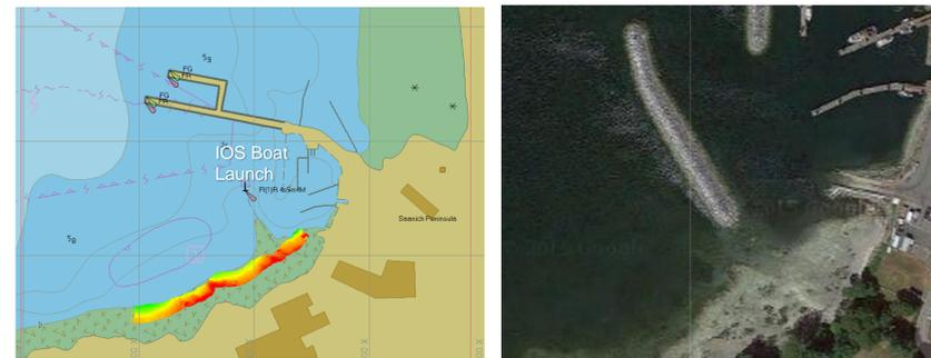
To test bathymetric performance for both flat and complex seabed geometries, a near shore survey was conducted. Binned bathymetry and variance results were compiled along with individual sounding examples at different swath distances.
