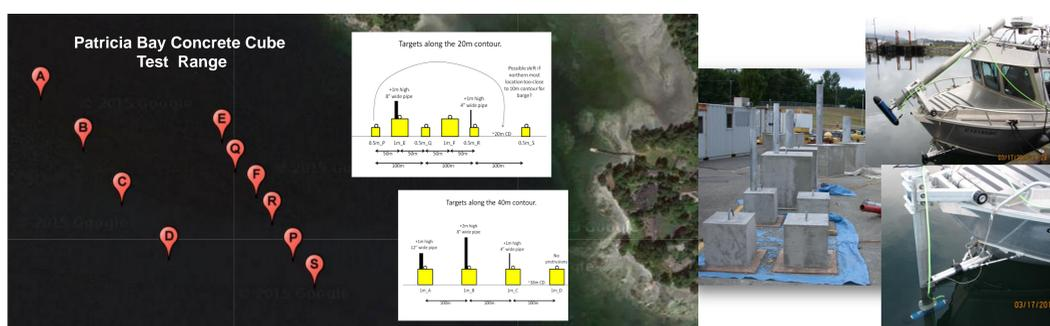
To test detection of small-scale features, a survey was conducted of the Patricia Bay Concrete Cube Test Range using the CHS vessel *Shoal Seeker* with the **3DSS-DX-450** bow mounted. Binned bathymetry and 3D point cloud results were compiled.
