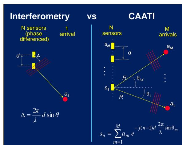
CAATI extends conventional phase based interferometry to multiple simultaneous angles of arrival.
